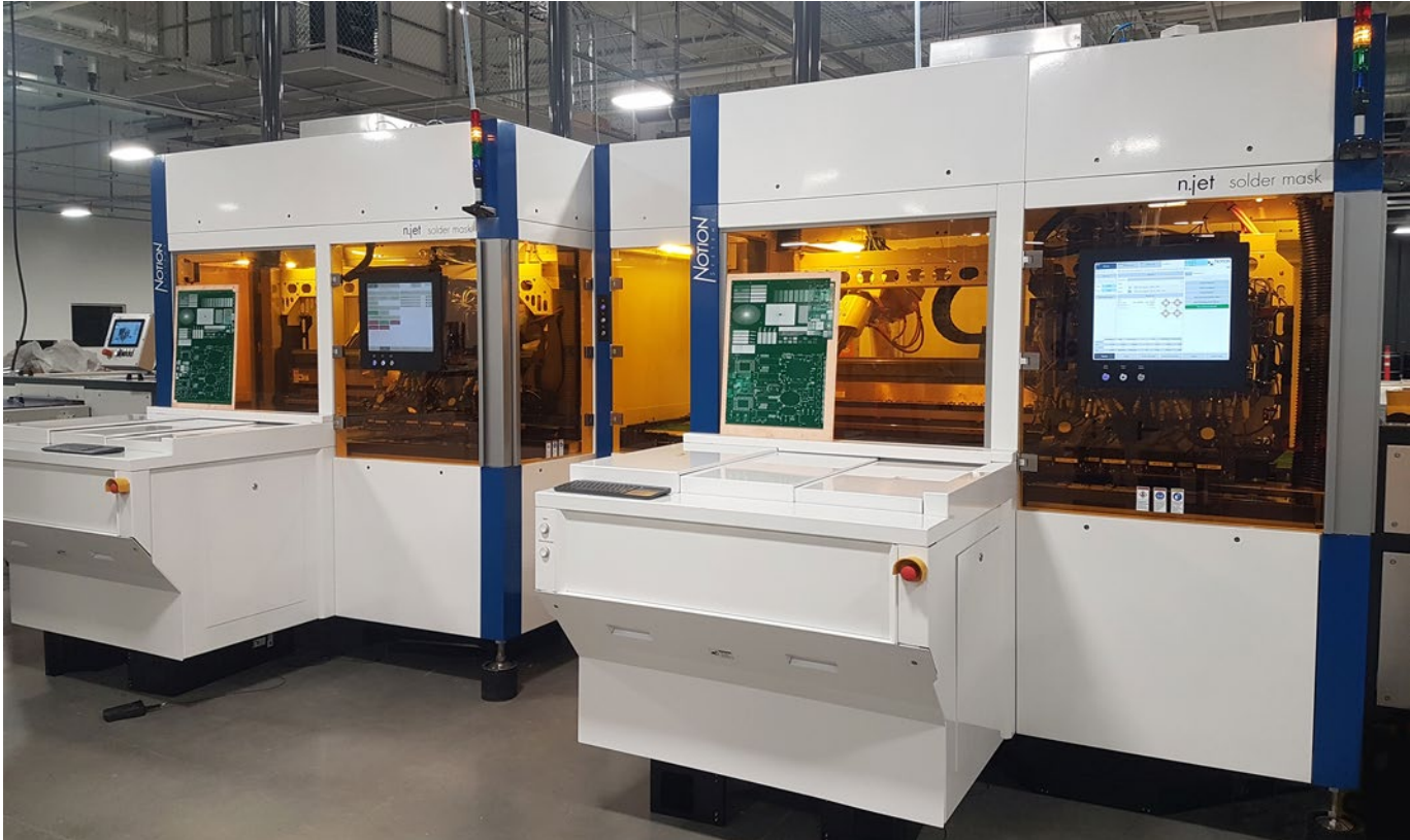
Notion Systems' n.jet technology saves multiple process steps, large investments in valuable space, energy, and labor. This completely digital process also uses UV-curable inks instead of solvent-based inks, which has far reaching effects on the environment.
