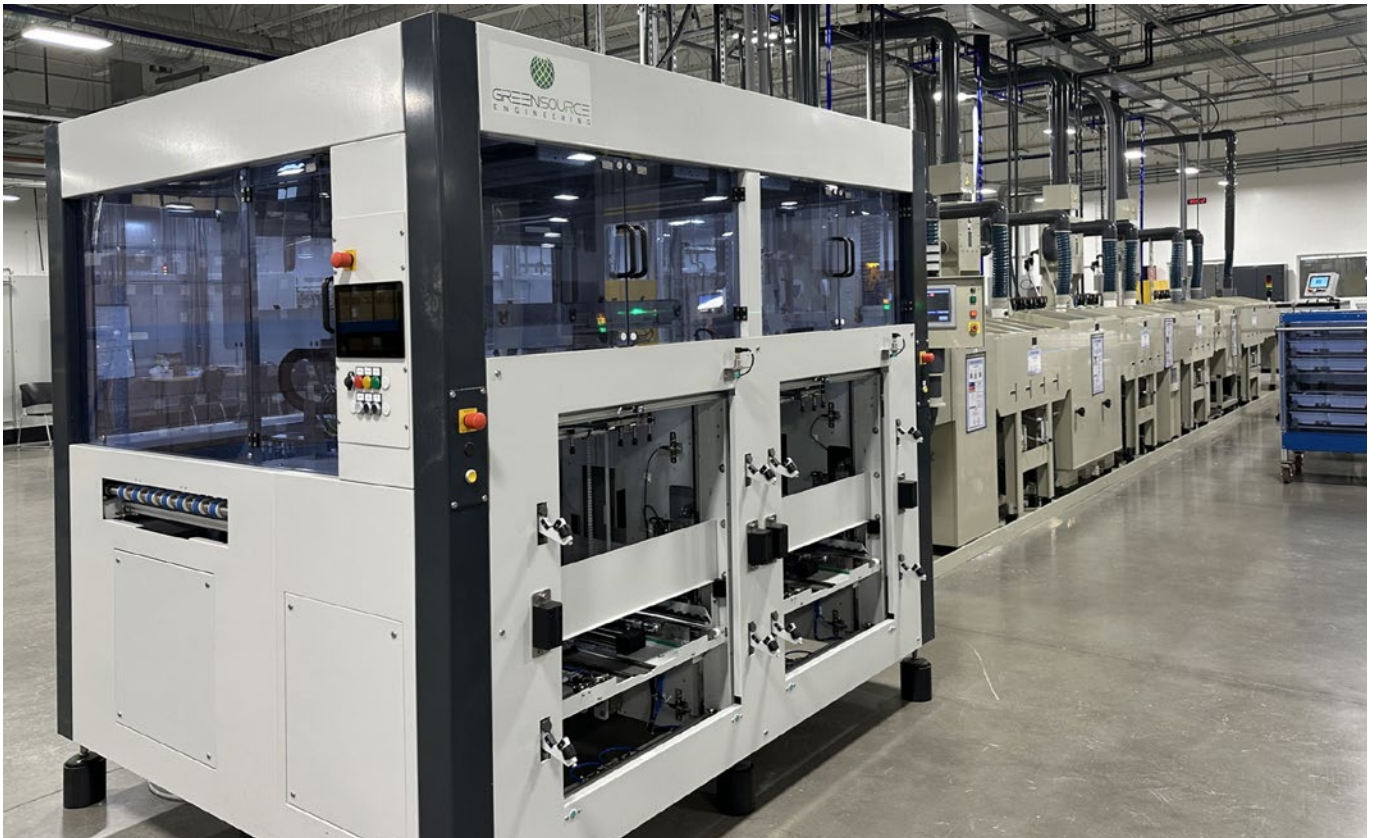
From left: GreenSource Engineering (GSE) double loader, photoresist strip line, GSE unloader.
