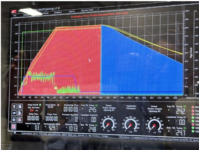
InduBond lamination press profile data.
