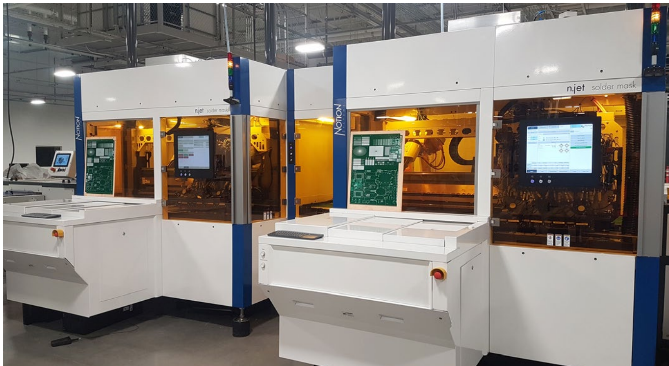
Notion Systems' n.jet technology saves multiple process steps, large investments in valuable space, energy, and labor. This completely digital process also uses UV-curable inks instead of solvent-based inks.
